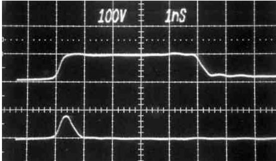
AVR-E4-C-P, at maximum & minimum pulse widths.
